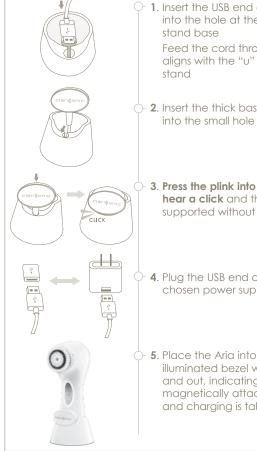
○- 1. Insert the USB end of the pLink charger into the hole at the very center of the
